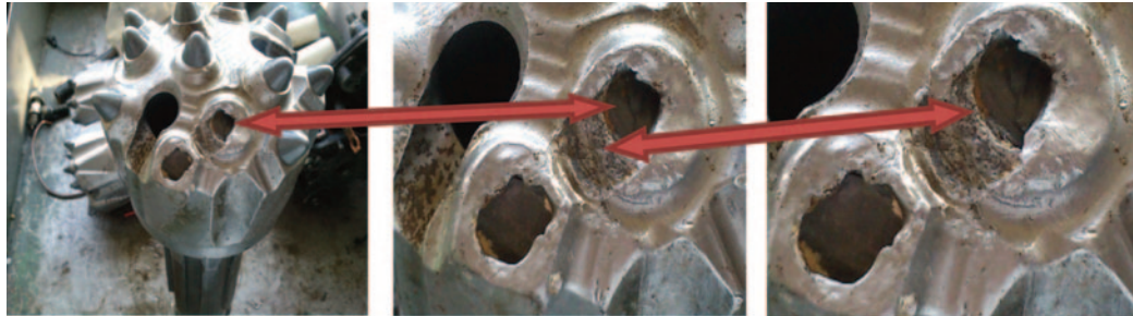
Figure 6. Appearance of a DTH hammer drill bit, with carbides loss points, after drilling 384 m
