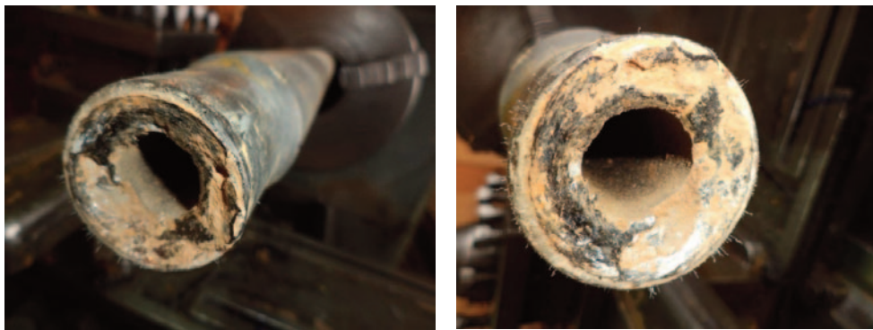
Figure 3. Appearance of the drill rod after fracture (limestone quarry "Vijenac")
